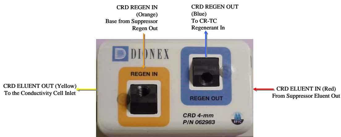
FIGURE 1 CRD Basic Plumbing
