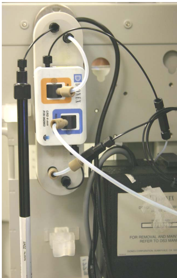
FIGURE 6 CRD Installed in the System
