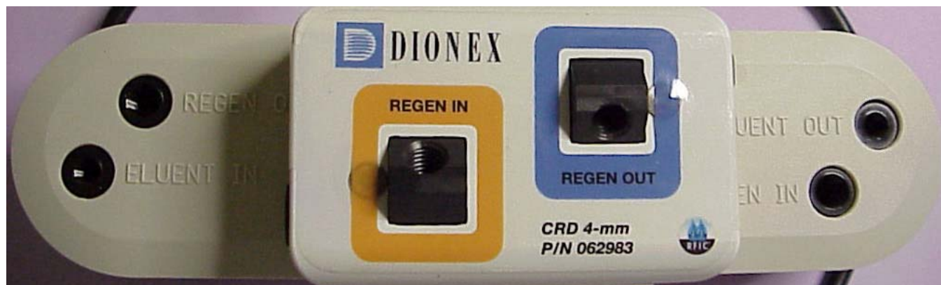
FIGURE 4 CRD Mounted on SRS
